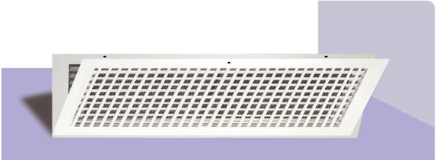
>> The fresh air grille is composed of a return grille that is either an egg crate grille or fixed blade grille which is fixed to a frame that contains a filter by means of steel hinges.
